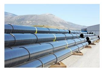
The agreement covers approximately 76 km of 8" - 16" High Frequency Welded (HFW) linepipe with external 3-layer polyethylene coating. The HFW pipes will be manufactured and coated at Corinth Pipeworks' facility in Greece and delivered to Mozambique within 2022.
