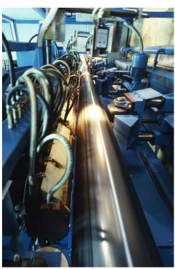
The steel pipes will be manufactured at Corinth Pipeworks' facilities and will include three-layer polyethylene external and epoxy internal coating, applied at the same location as the pipe manufacturing, at the Thisvi plant, in Greece.
