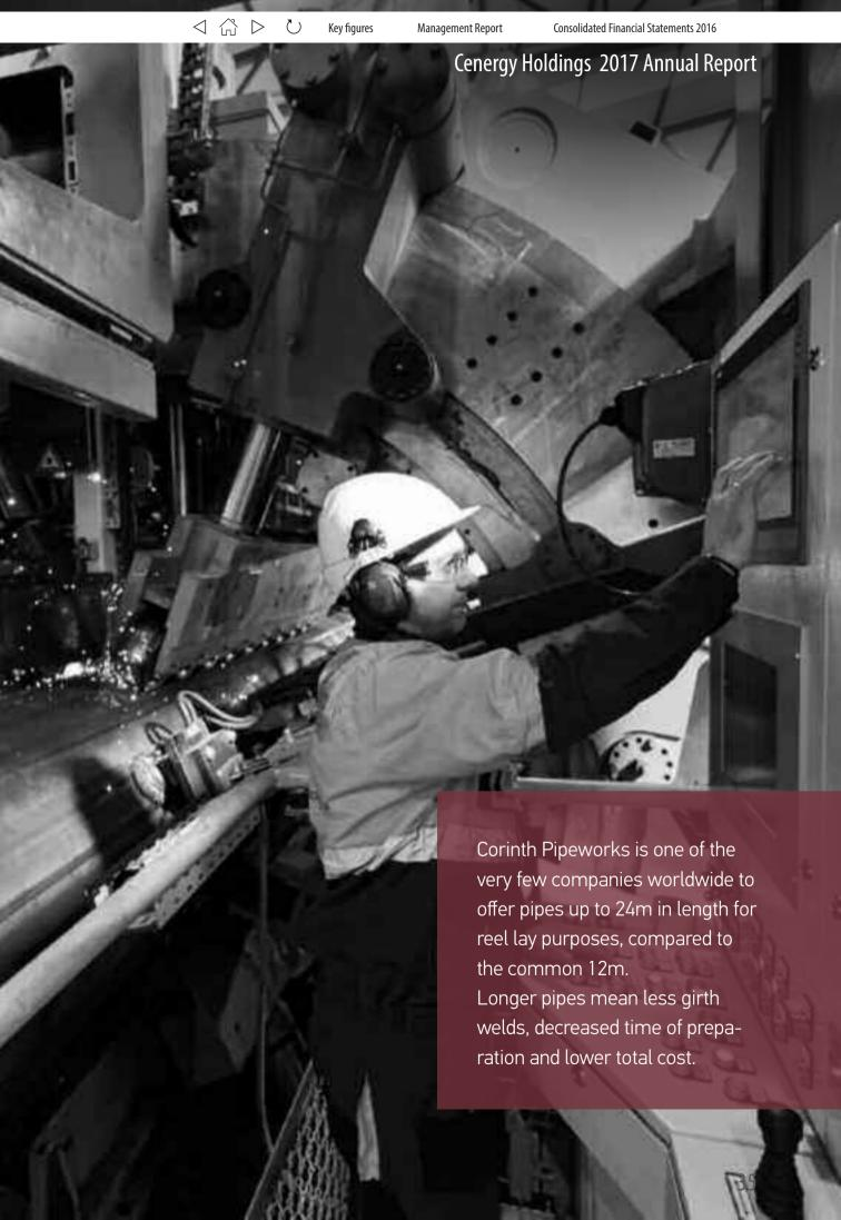
Corinth Pipeworks is one of the very few companies worldwide to offer pipes up to 24m in length for reel lay purposes, compared to the common 12m. Longer pipes mean less girth welds, decreased time of preparation and lower total cost.
